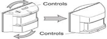
If the sensor pops out of the ball joint, loosen the clamp screw and push the sensor back into the ball joint. Tighten the clamp screw when done.
