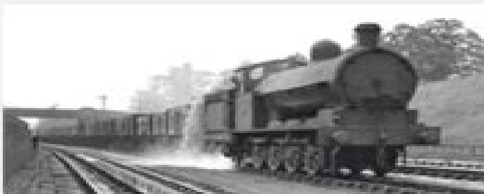
LMS class 'D' 0-6-0 No. 2220 takes coal from Buxley brought with a Down train of coal empties on August 23, 1926. This engine was rebuilt from a class 'K' compound in May 1926 and was further rebuilt as LMS No. 2024 to class 'GJ' in September 1927. It was 'upgraded' to 'Gda' in September 1944, and was withdrawn in November 1944 from Wigton Springs Branch. In one form or another it had given almost 60 years of service, having first been built at Crewe in February 1895. R.A. HARRISON/RAIL ARCHIVE STEPHENSON
