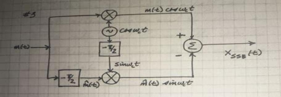
Using the diagram given above and setting  $m(t) = Cos(\omega_m t)$  verify that the output of the 55B generator given above is indeed an 55B signal. Which sideband is generated, USB or LSB. (Do wath)
