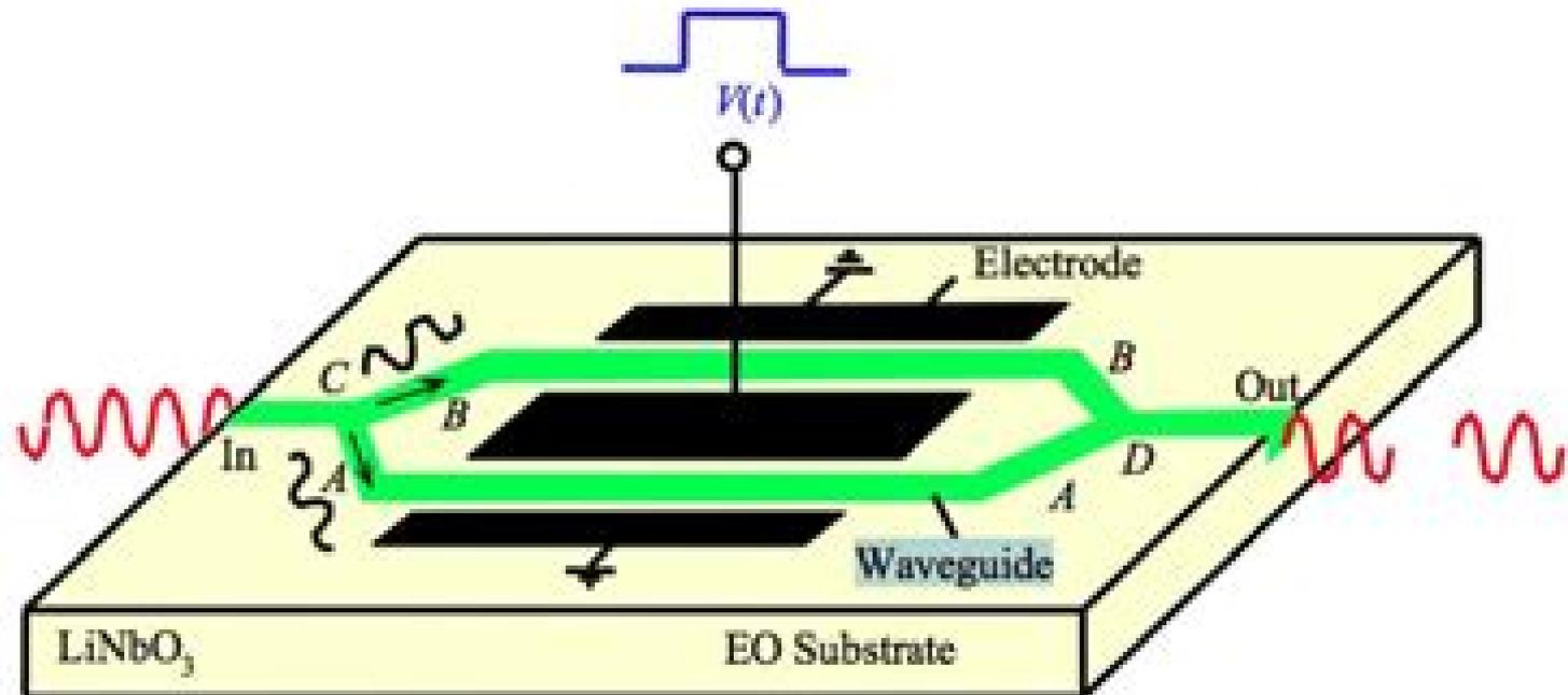
The input light is split into two coherent waves  $A$  and  $B$ , which are subject to different phase shifts induced by the applied voltage, and then the two are combined again at the output.
