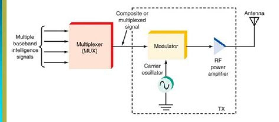
Figure 1-11: Multiplexing at the transmitter.
