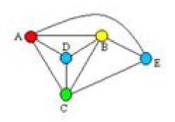
Planar graph - a graph drawn in a plane without any of its edges crossing or intersecting
