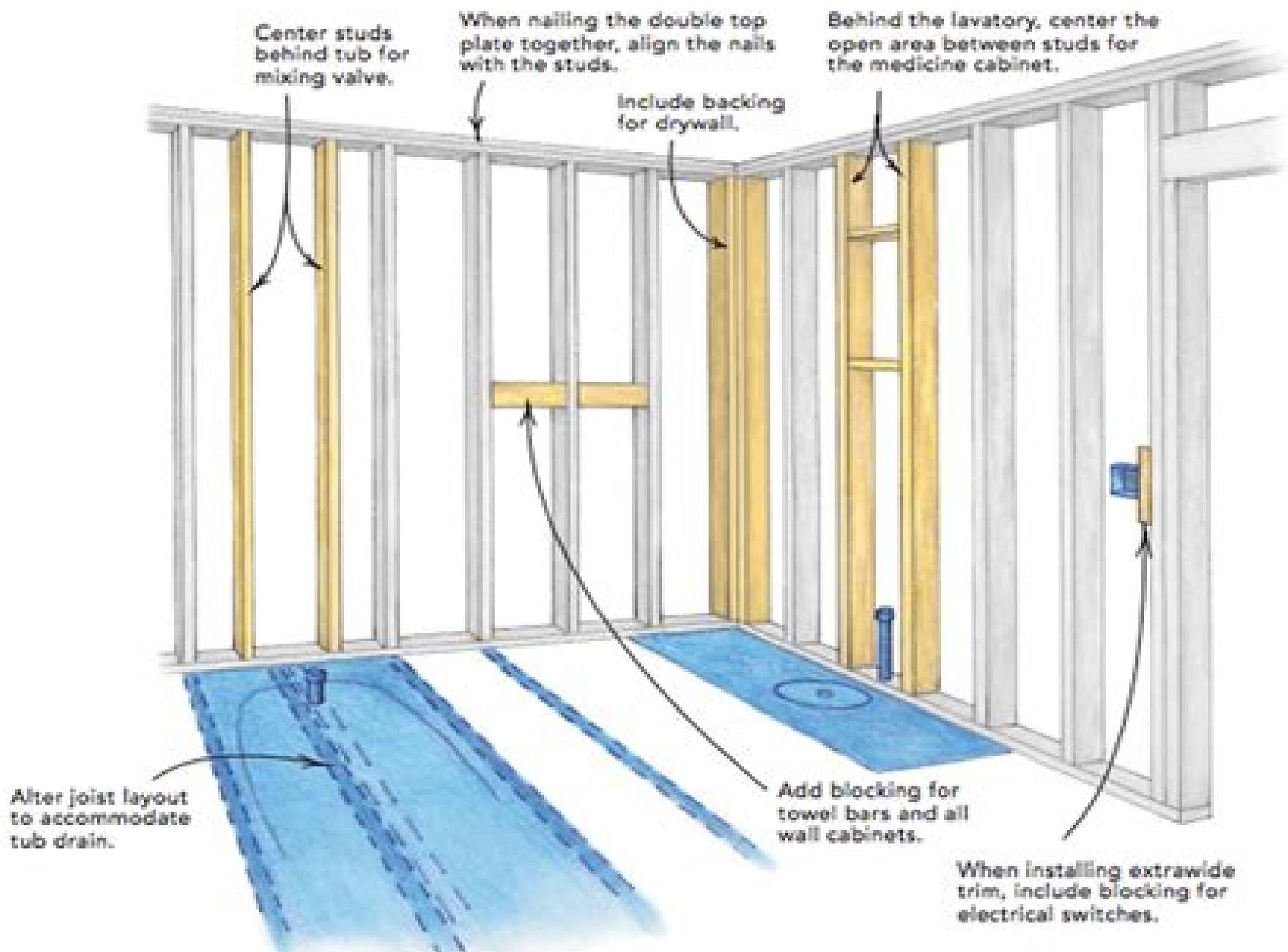
Center studs behind tub for mixing valve.
