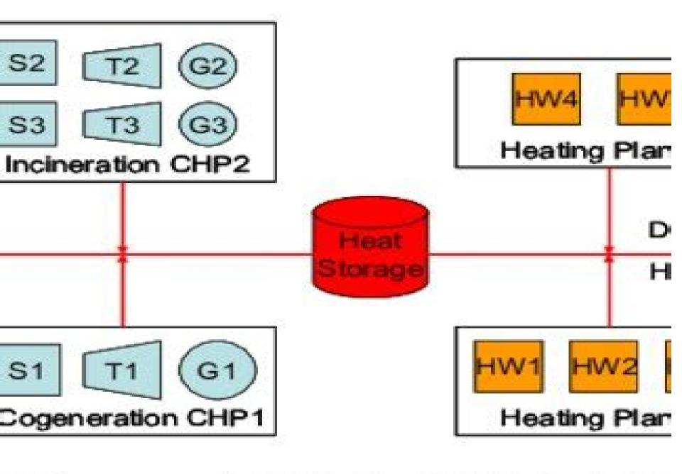
S-Steam generator | T-Turbine | HW-Hot water bo
