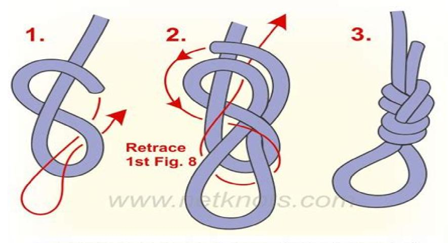
This knot can also be tied by tying a Figure Eight Knot with doubled line at the end of a rope (Fig. 1. with doubled line and don't come back through bottom loop.) It is faster but cannot be used if tying onto a fixed object. A single Figure Eight also makes a good "Stopper Knot" at the end of a rope.
