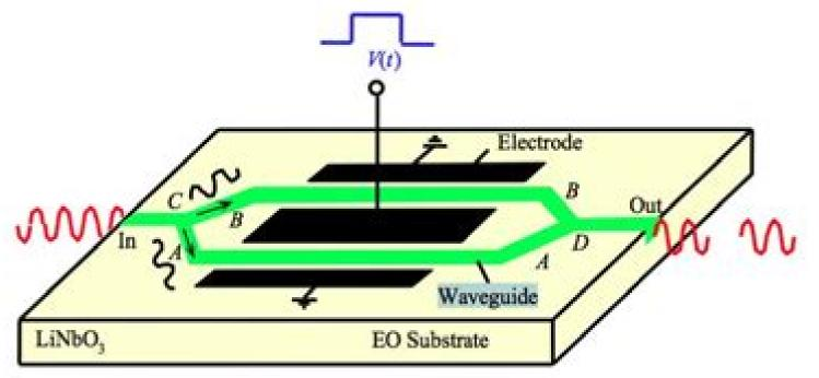
The input light is split into two coherent waves A and B, which are subject to different phase shifted induced by the applied voltage, and then the two are combined again at the output.
