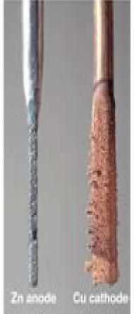
overall reaction:  $Zn(s) + Cu^{2+}(aq) \rightarrow Zn^{2+}(aq) + Cu(s)$
