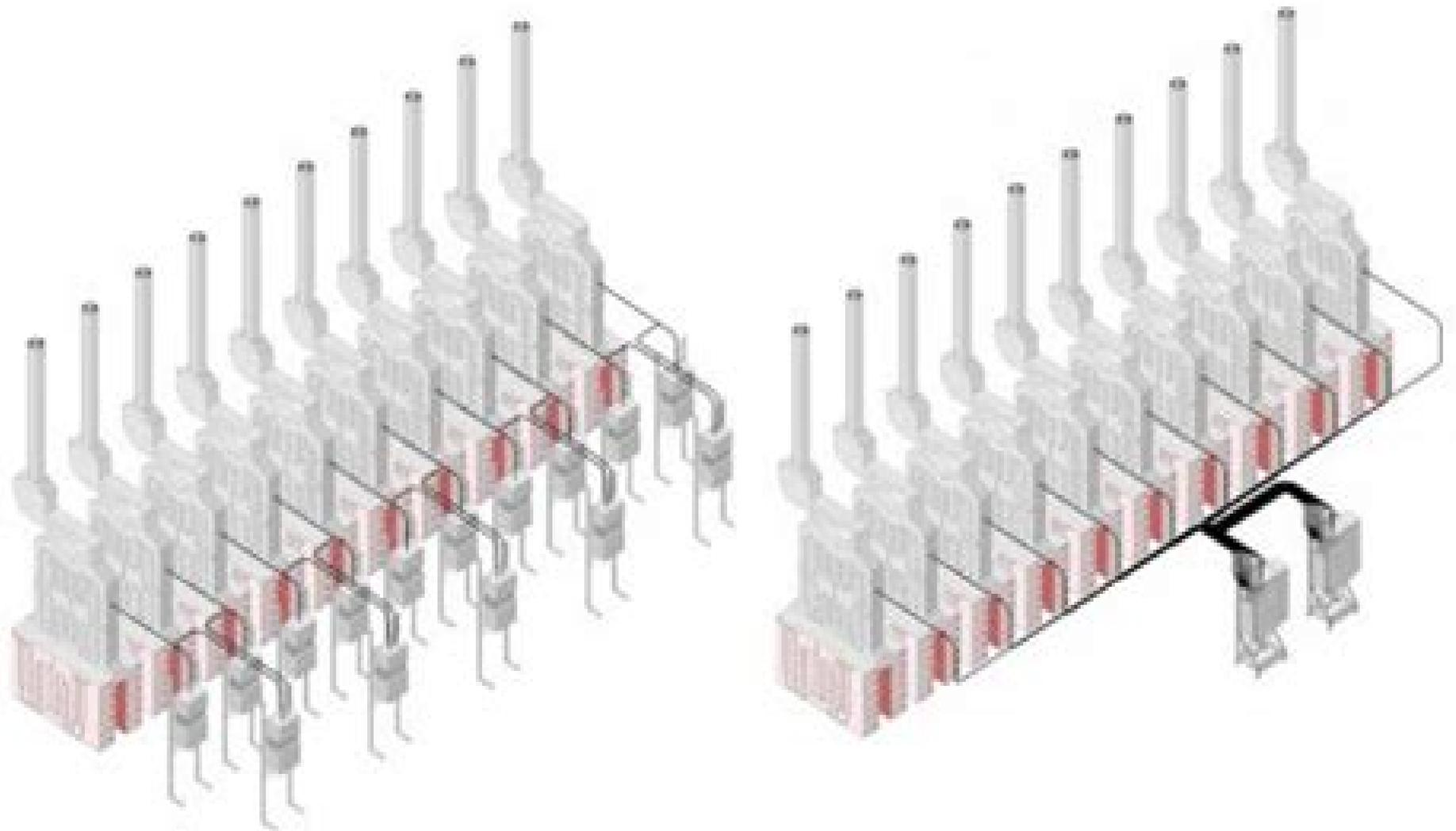
Two Process Mass Spectrometers (right) used in place of 15 gas chromatographs (left) on ethylene turnâ€ces for effluent gas analysis.
