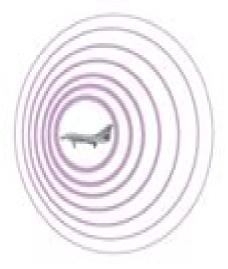
An aircraft in flight creates a series of pressure waves that travel outward in all directions and perceived as sound
