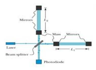
NASA and the European Space Agency (ESA) were jointly developing a space-based probe called the Laser Interferometer Space Antenna (LISA) which was to measure fluctuations when a gravitational wave passes.
