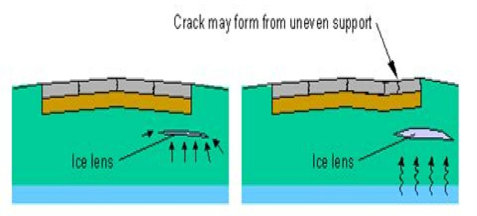
Ice lens begins to form from free moisture in the soil lce lens grows as it is fed from water by capillary movement through frost susceptible soil causing pavement to heave and sometimes crack
