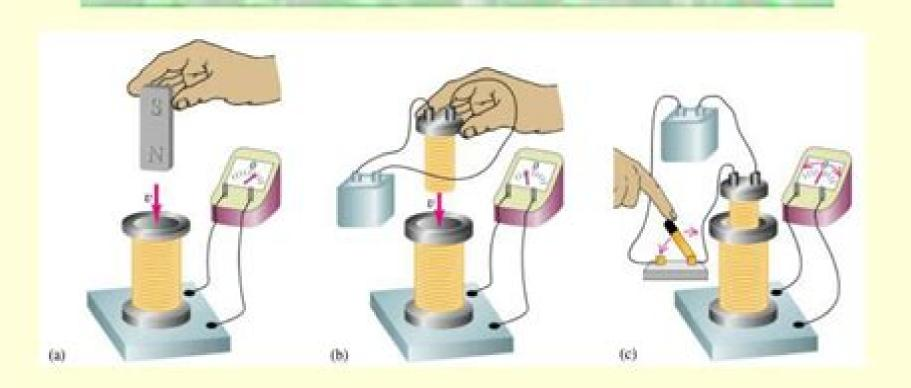
emf is induced in a conductor placed in a magnetic field whenever there is a change in magnetic field.
