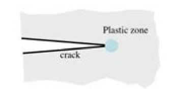
Applies when non-linear deformation is confined to a *small* region surrounding the crack tip Effects of the plastic zone negligible, linear asymptotic mechanical field (*see eqs 4.36, 4.40*).
