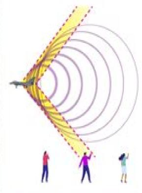
Eventually the waves merge into a shock wave. A person on the ground hears a boom when the shock wave crosses his location.
