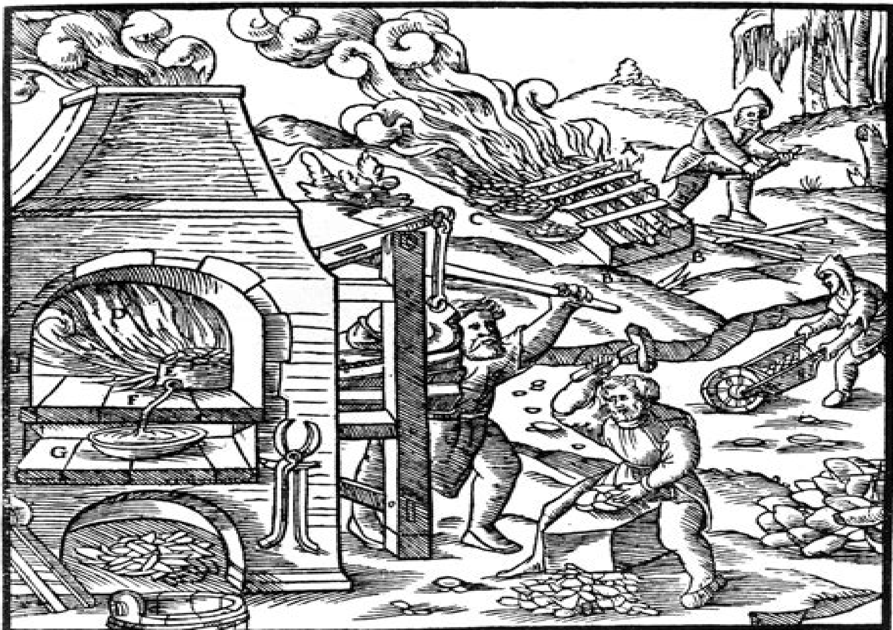
A—WOOD. B—BRICKS. C—PANS. D—FURNACE. E—CRUCIBLE. F—PIPE. G—DIPPING-POT.
