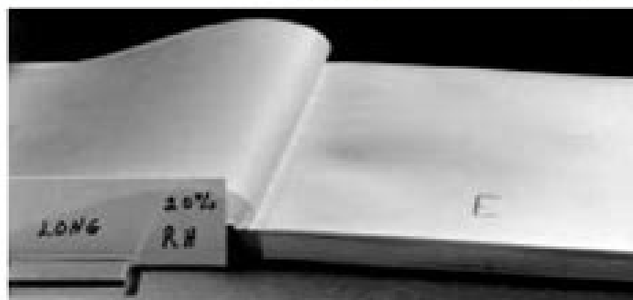
Figure 10. Curves for all four laboratory cases, at 20% RH, as shown above, all identical. Curves are left for unprocessed, and curves are right for processed.
