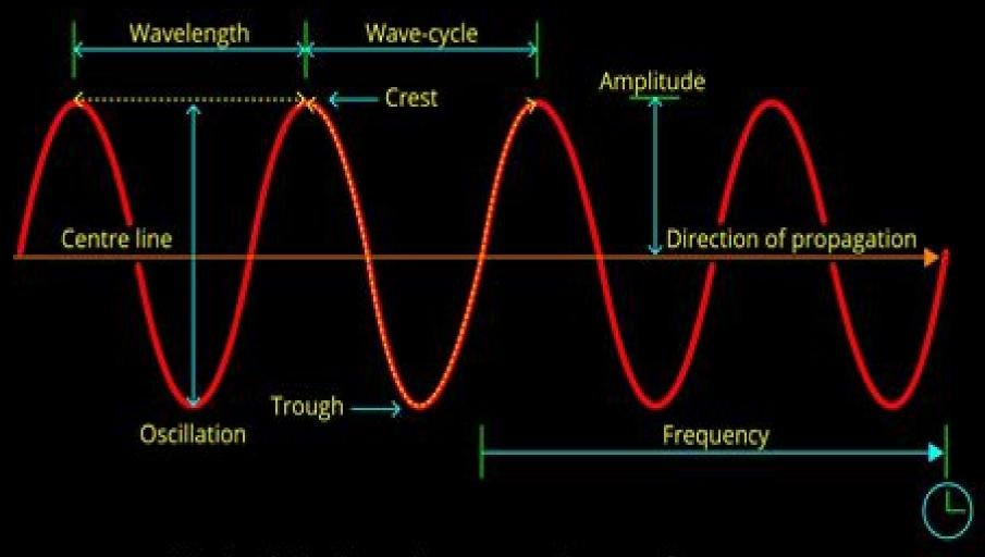
Wavelength: The distance between successive crests of a wave Frequency: Wave cycles passing a given point in a given period of time Amplitude: Measured between the crest and the mid-point of a wave Velocity: Speed and direction of propagation
