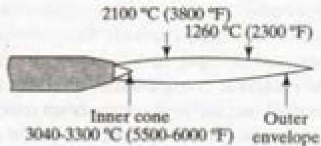
(c) Carburizing (reducing) flame
