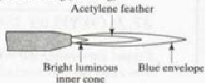
(c) Carburizing (reducing) flame
