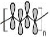
p orbitals along the backbone, each one contains one electron Overlapping of 3n atomic p orbitals generates 3n molecular orbitals, 3n/2 are occupied by 3n electrons, 3n/2 are empty
