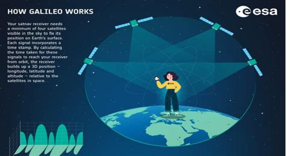
All Galileo satellites transmit at the same frequency bands. To let the receiver distinguish between them, each satellite has its own code embedded in the signal. The receiver compares the received code to local replicas it has stored – this also helps with acquiring what is a very weak signal – equivalent to a torch light shining across a continent.
