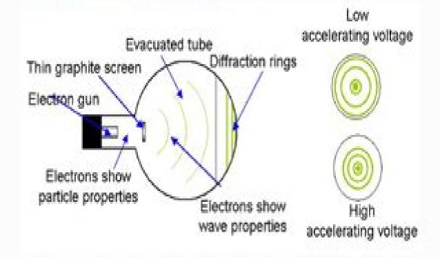
Electrons fired at a thin crystal structure of graphite (carbon) produced an interference pattern of bright and dark rings on a fluorescent screen Particles were behaving like waves- more about this later.
