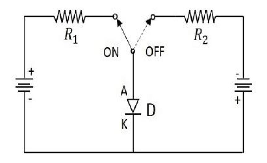
Switching circuit using Diode
