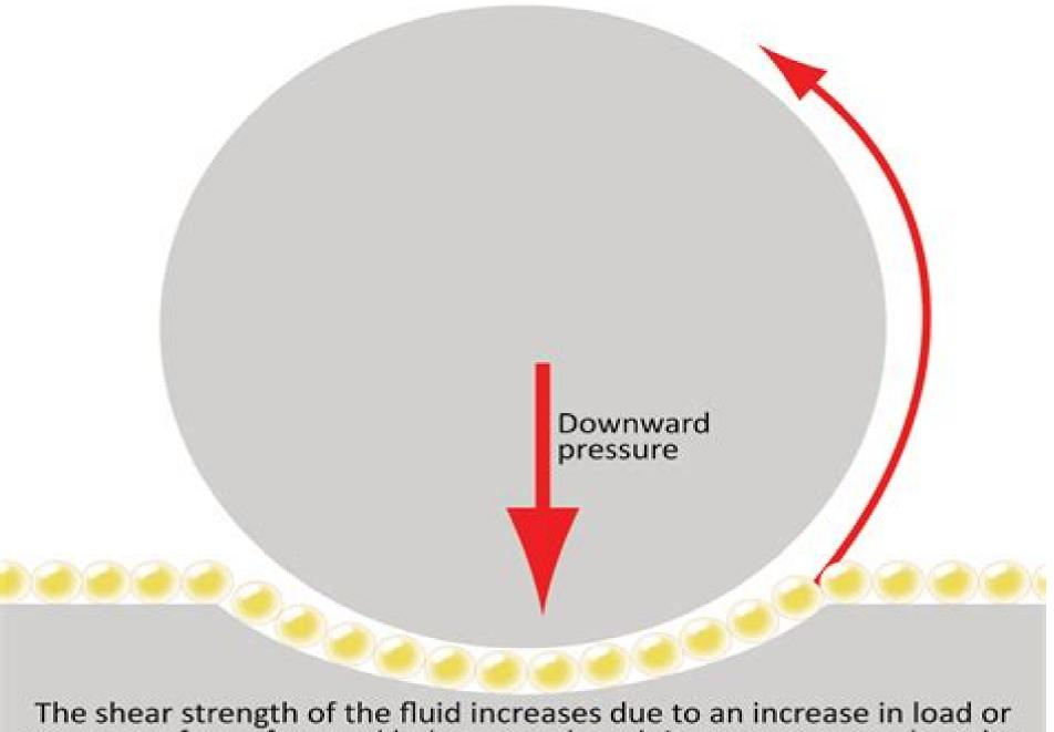
The shear strength of the fluid increases due to an increase in load or pressure of a surface and behaves as though it were stronger than the metal surface it acts against, thus causing the surface to deform.
