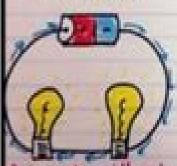
A break will stop the whole current Parallel Circuit (more than one path)
