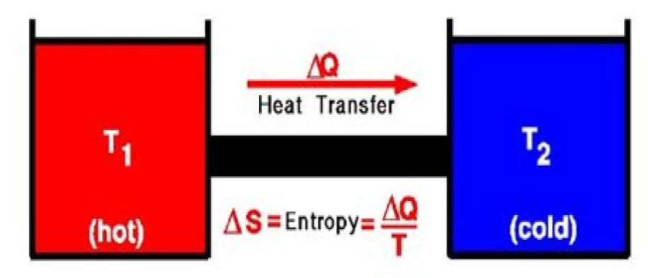
There exists a useful thermodynamic variable called entropy (S). A natural process that starts in one equilibrium state and ends in another will go in the direction that causes the entropy of the system plus the environment to increase for an irreversible process and to remain constant for a reversible process.
