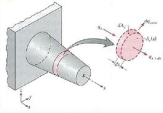
$$\frac{d^2T}{dx^2} + \left(\frac{1}{A_c}\frac{dA_c}{dx}\right)\frac{dT}{dx} - \left(\frac{1}{A_c}\frac{h}{k}\frac{dA_s}{dx}\right)(T - T_{\infty}) = 0 \qquad \text{Eq. (3.61)}$$
