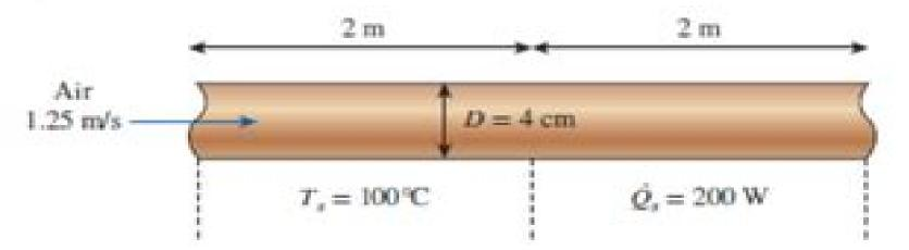
Determine the air temperature at the 2 m length.
