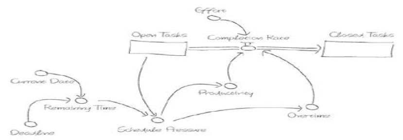
As noted in the previous section, this stock and flow diagram is just a visual notation for a mathematical model of the system that can be used to simulate the system's behavior using computer software. In these mathematical models, stocks and flows are represented by integral equations, converters are represented by functions of their input and/or time. In most cases, these integral equations cannot be solved analytically but instead are approximated using numerical integration.
