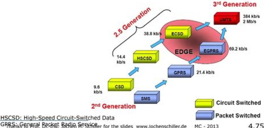
GRRS: General Backet Radio Sestinger for the slides www.jochenschiller.de EDGE: Enhanced Data rates for GSM Evolution
