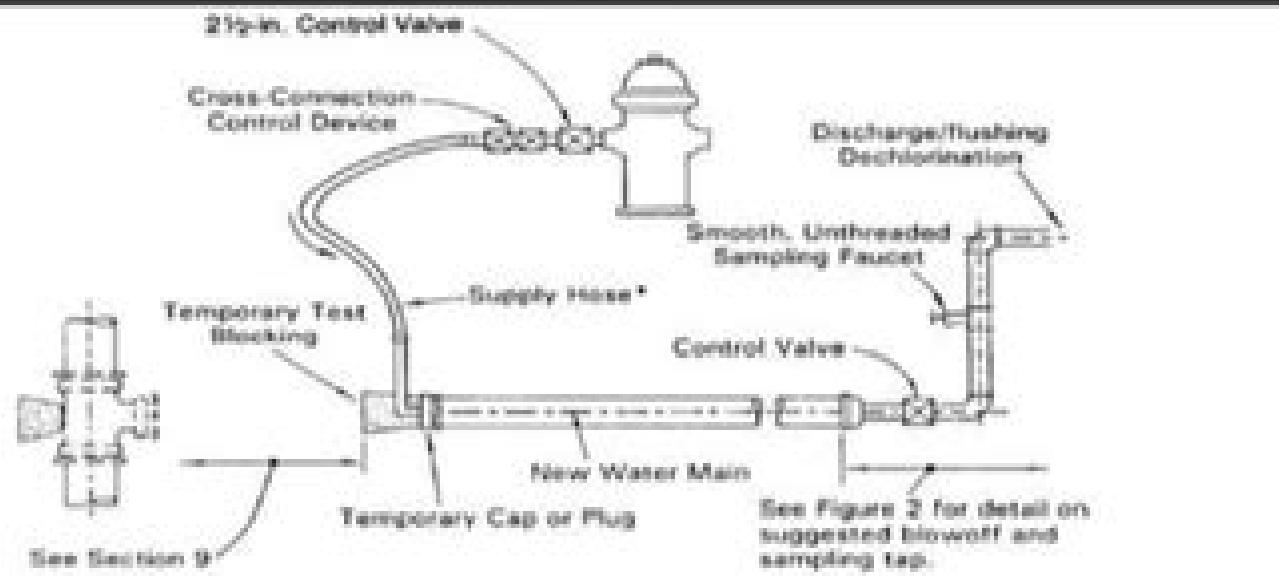
\*Clean potable-water hose only. Size and number of taps per Table 3. This hose must be removed during the hydrostatic pressure test.
